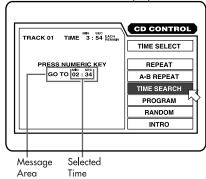
Use the CURSOR buttons ▲/▼ to move to [TIME SEARCH], then press ENTER 22. "GO TO" appears in the message area. The color of [TIME SEARCH] changes. Use the numeric buttons (0 - 9) (13) to enter the time. The specified time appears in the message area. Press the ENTER button (22). The RDV-985 starts playback at the selected time.
